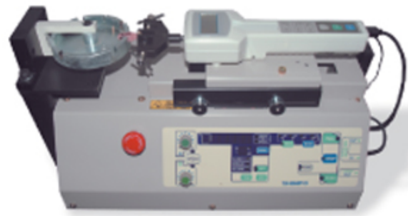
Special testing equipment to measure the quality of bondability
